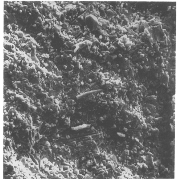
Figure 25 A scanning electron micrograph of a fracture surface of the whiskers-reinforced alumina specimen. The silicon carbide whiskers are 10 \mu\text{m} \times 0.7 \mu\text{m} in size (courtesy of D. Kupperman, Argonne National Laboratory).
